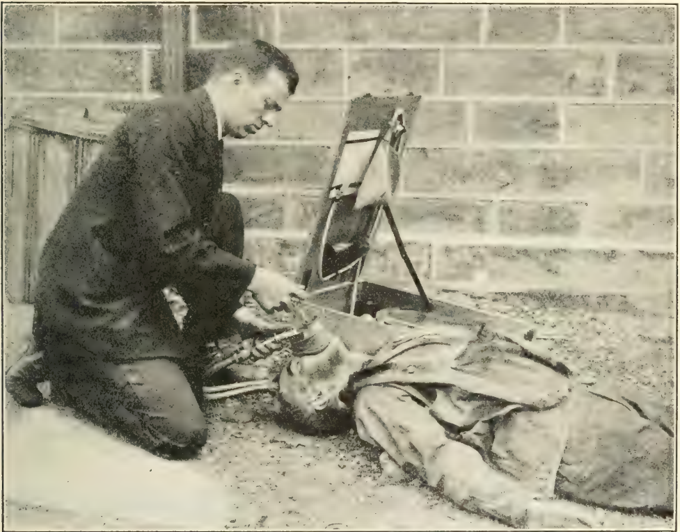
The Pulmotor, the Famous Resuscitating Device, Being Used in Reviving an Asphyxiated Miner
